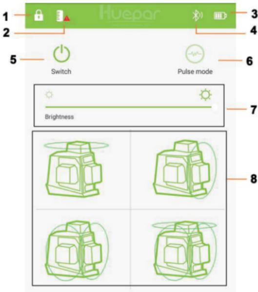
1. Smart Pendulum Lock Status: When the laser tool is turned on in manual mode, icon 1 will be displayed; when turned on in self-leveling mode, icon 1 will disappear.
